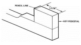
Figure 6-4. Key Pedestal - Pencil Line Dimension
