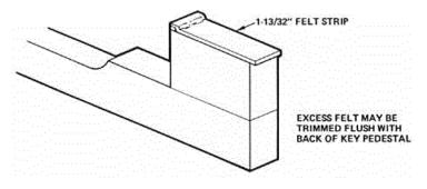
Figure 6-6. Key Pedestal - Felt Modification Complete
