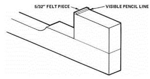
Figure 6-5. Key Pedestal - 5/32" Felt Piece Mounted
