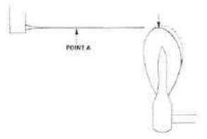
Figure 9-2. Tear-Drop Hammer Head - Reshaping to Striking Line
